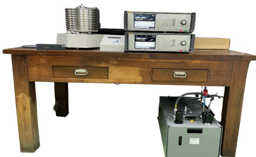
Nitrogen Operated PUC, Range 1000 bar, having uncertainty \pm 0.005\% of Rdg.
