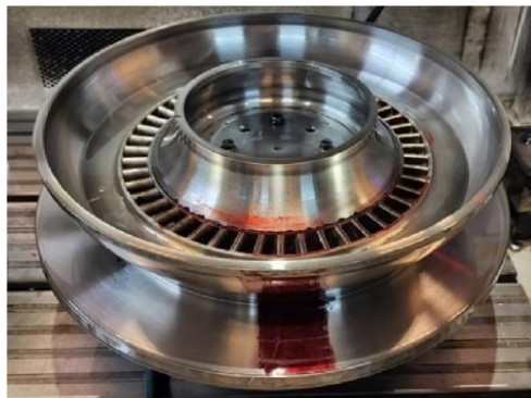
1100 -72 Nozzle block EDM machining for CE20 (cryogenic engine) Turbo Pump assembly for ISRO LPSC through M/s MTAR.
