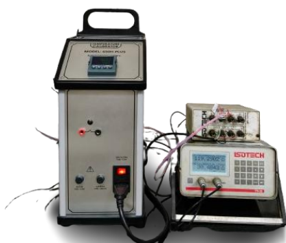
CALIBRATION OF PRT SENSOR BY COMPARISON
